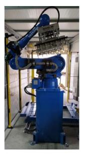
This is because the reducers do not require maintenance, and endless screws, drive belts, and limit switches on the axes, elements that require increased replacement and adjustment costs, are omitted. A robotic gripper was added to this arm, capable of transporting sacks from the pick-up point to the pallet without altering the product's geometry or causing damage.
